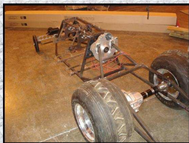
The Completed rolling chassis of the frame weighs only 225lb.
